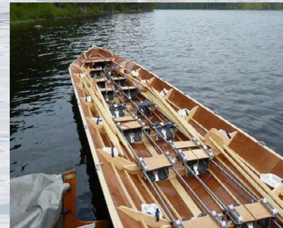
Sliding seat system with grooved rollers sliding on round stainless steel guide rails. Rugged, comfortable and low maintenance design. Picture courtesy of Puuvenepiste Oy
