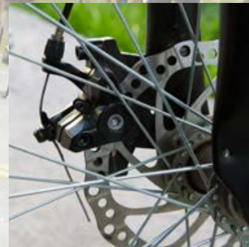
Disk brake rotor for Mountain Bike. AISI 410 -EN 1.4006 stainless steel
